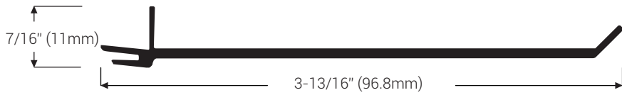
ECE3JCC Jamb cover clad (aluminum)
