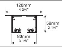
Finish: Max. Door Weight: Min. Door Thickness: Carriage Pack: Clear anodized 500kg 1100lb 40mm 1-9/16" M10 only
