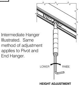
A. Close leaves and adjust the door height to achieve an equal gap between the top of the leaves and the track (a 9 [0.35"] gap is recommended).
