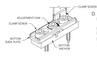
D. Replace the Bottom Pivot Bolt and tighten to Bottom Slide Plate. Mark the position of the Bottom Slide Plate.
