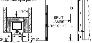
5. Fasten bottom door guides so that door stays in center of pocket, yet travels easily without binding.
