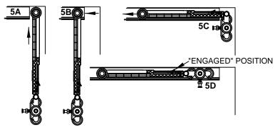
INSERT 1060 Actuator Arm into track, with back of Actuator Arm 1-1/2" (38mm) from each end of track, (24" doors: Actuator will be flush with end of track). HAND TIGHTEN (do not use power drill) Actuator Arm on track legs. Check to make sure Arm remains straight in track.
