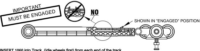
INSERT 1060 into Track. (Idle wheels first) from each end of the track.
