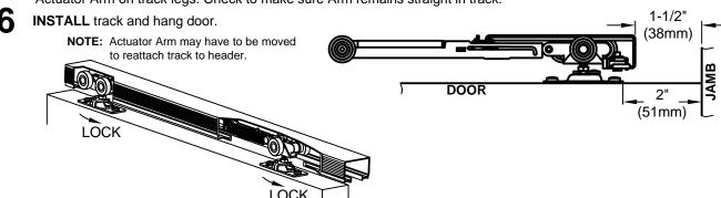
SLOWLY slide door toward Jambs, checking to make sure door touches Jamb, if not. Slide door away from Jamb and readjust Actuator Arm. Slowly close door again, checking to make sure soft close is working properly. Once confirmed, being using door normally.
