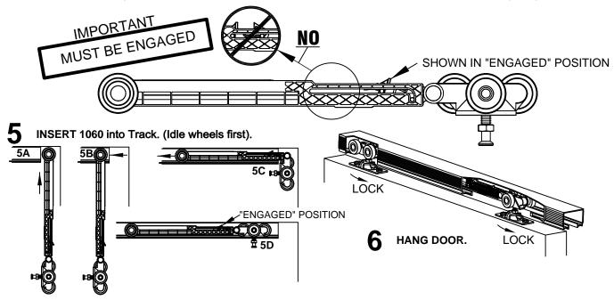
SLIDE door away from end of track (check to make sure all track screws are flat against track) and install 1060 Actuator Arm into track, with back of Actuator Arm 2-1/4" (57mm) from Jamb. HAND TIGHTEN (do not use power drill) Actuator Arm on track Check to make sure Arm stayed straight in track. Slowly close door, checking to make sure door touches Jamb, if not. Slide door away from Jamb and
