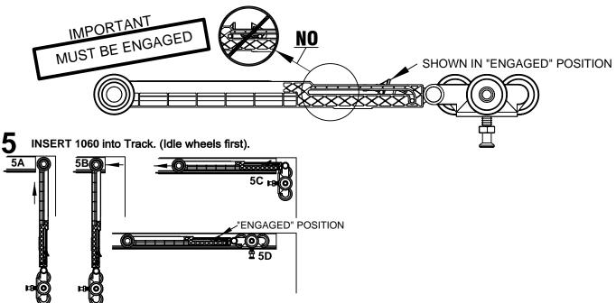
**INSERT** 1060 Actuator Arm into track, with back of Actuator Arm 1-1/2" (38mm) from end of track, (18-24" doors: Actuator would be flush with end of track). HAND TIGHTEN (do not use power drill) Actuator Arm on track legs. Check to make sure Arm remains straight in track.
