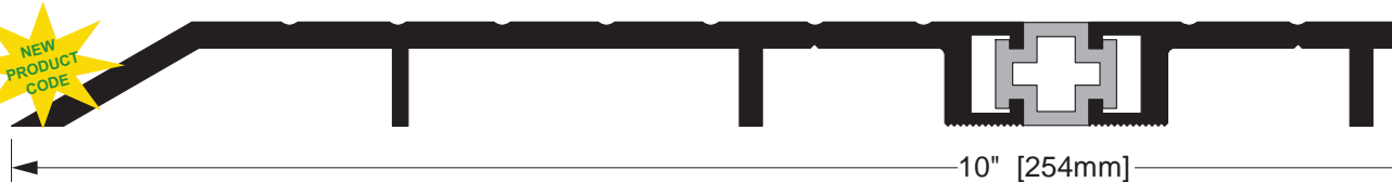
CT-410 EXTRUDED ALUMINUM WITH RIGID P.V.C.
