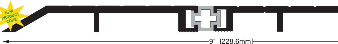
CT-409 EXTRUDED ALUMINUM WITH RIGID P.V.C.
