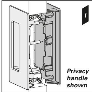
c) Repeat the process with the other side handle, taking care to line up the alignment pins with the two holes in the side handles and the third hole in the snib button (only applies to privacy handles) (**diagram f**).
