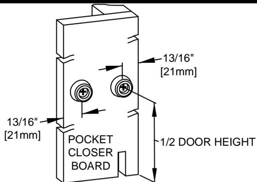
**16 FASTEN** 1513 Bumpers to back of Pocket Closer Board 1/2 the door height from floor. 13/16" (421m) from each edge.
