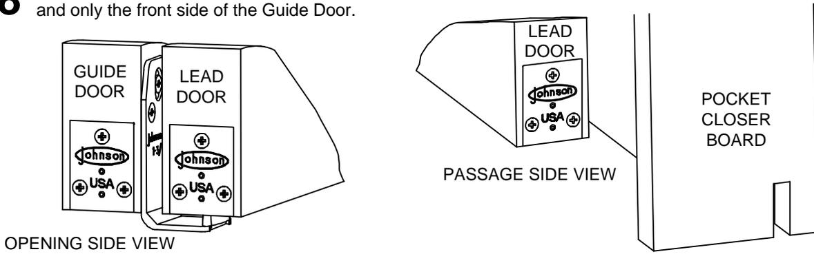
**19 SLIDE** 1155 Stop into Guide door track and adjust until the back edge of the Pocket Closer Board on the guide door is flush with the front edge of the steel wrapped studs.
