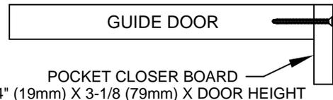
**8 ATTACH** Pocket Closer Board to back edge of Guide Door.
