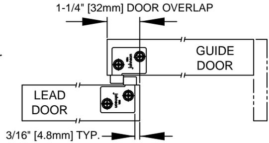
**14 A/Attach** door plate 1121 on top of door 2" (50mm) from each edge with lock tab on same side.
