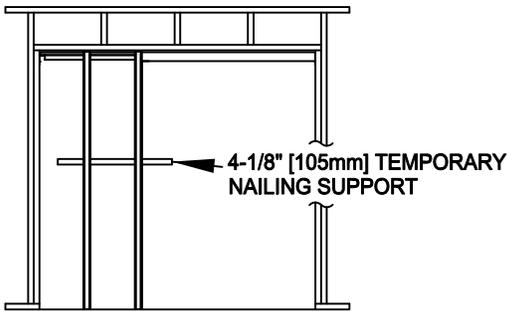
**6 APPLY** desired wall material. Wall material is bought clear to edge of opening. **WARNING:** Use screws no longer than necessary. Screws must not protrude into pocket or doors will be damaged. To provide a firm surface, slip a 4-1/8" (105mm) wide board between Split Studs temporarily.
