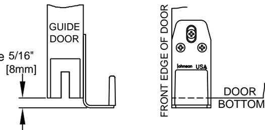
**13 ATTACH** 2054 Pull Catch to top front edge of Guide Door and top rear edge of Lead Door.
