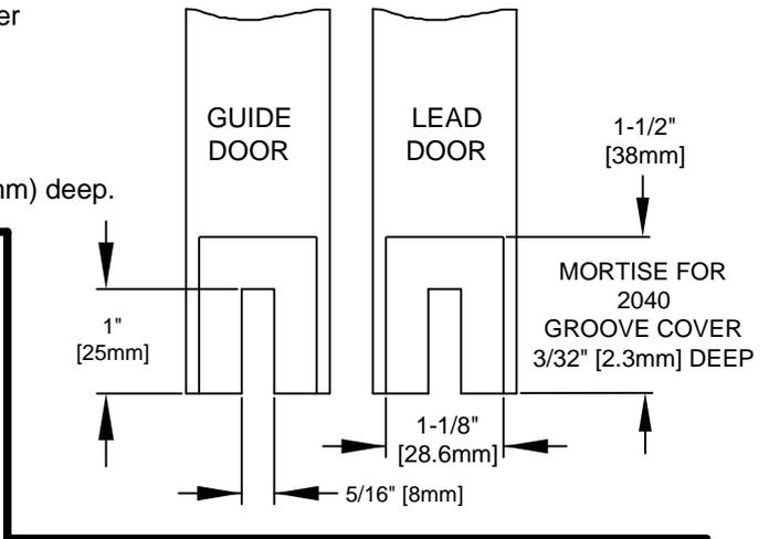
**11 REMOVE** Pocket Closer Board from Guide Door and seal all edges and faces of doors and pocket closer board with paint or sealer stain.
