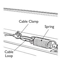
Adjust the adjuster nut to tension cable to eliminate sag. Lock off the lock nut.
