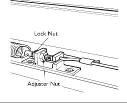
Position doors to be centered within opening. Tighten grub screws in cable collar. Test operation of system to ensure correct installation.
