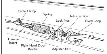
Fit adjuster bolt onto the right hand door bracket. Hook spring onto the adjuster bolt and hook cable loop onto the other end of the spring.
