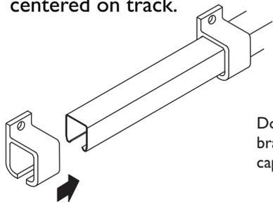
Do not install end brackets with end caps at this time.
