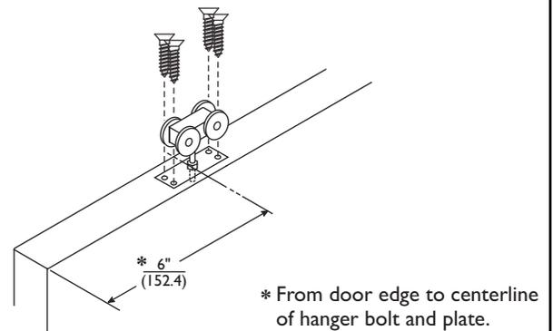
\* From door edge to centerline of hanger bolt and plate.
