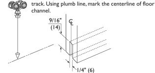
Attach a plumb line to hanger. Place hanger inside
