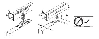
8. Position and secure retaining stop.
