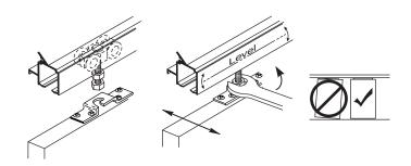
8. Position and secure retaining stop.
