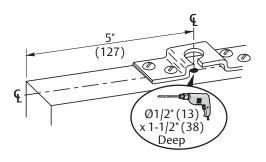
3. Insert hangers and retaining stops.
