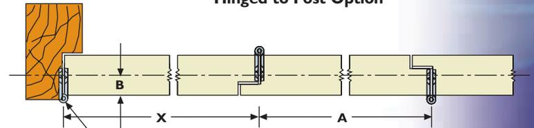
Note: Butt hinges on posts are not offset
