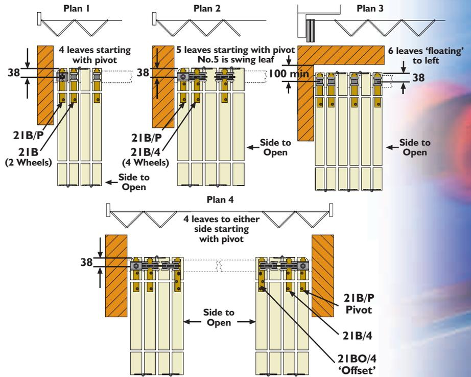
Note: Hangers and guides are to be fitted to alternate leaves only.
