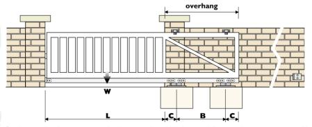
Min. weight of each concrete block for each roller = 1.7 x **W** (total gate weight with the track) (average concrete density: 2.6 to 2.8 kg/m³)
