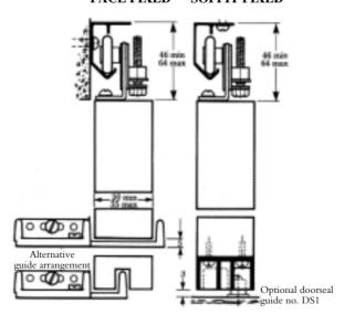
Easily fixed sliding doors for soffit or face fixing without drilling into door, and an easy-fix floor guide.
