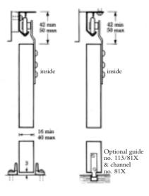
For a wide range of single leaf, wood or composite sliding doors, with face or soffit fixing top track and floor guides or optional bottom channel.
