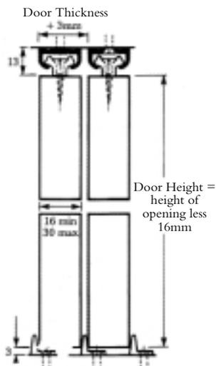
For lightweight wood or chipboard sliding doors eg. kitchens, bathrooms, serving hatches and built-in furniture where no bottom track is necessary. Silent and easy to fix, the doors can be simply removed when required.
